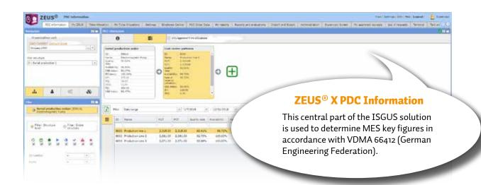
Within the PDC information screen, data and results are summarised and displayed in the target / actual-comparison. ZEUS® X PDC offers extensive filter options and a "drill-down"-function for all PDC criteria, in order to provide the user with an explanatory result. Analysis with just one simple click.
